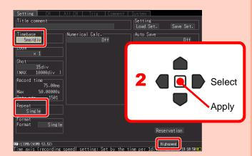
A 50 Hz measurement frequency is equivalent to 20 ms per cycle. When using the 5 ms/div time axis range and selecting to record 15 divisions, a 75 ms waveform can be monitored. (5 ms/div x 15div = 75 ms) This is equivalent to approximately 3.5 cycles.
