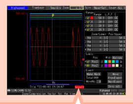
Press this key to display the "Scroll" icon on the bottom of the screen. (This key toggles between "Scroll" and "Cursor".)
