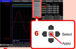
When the zoom ratio of the time axis is changed, the waveform printout will also zoom in or out accordingly.
